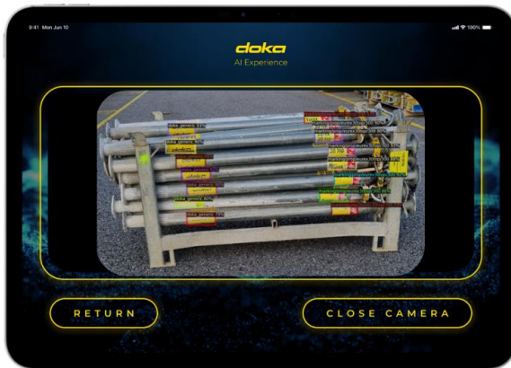
Figure 10 Identification and Counting of Formwork Products (Source: Doka)
